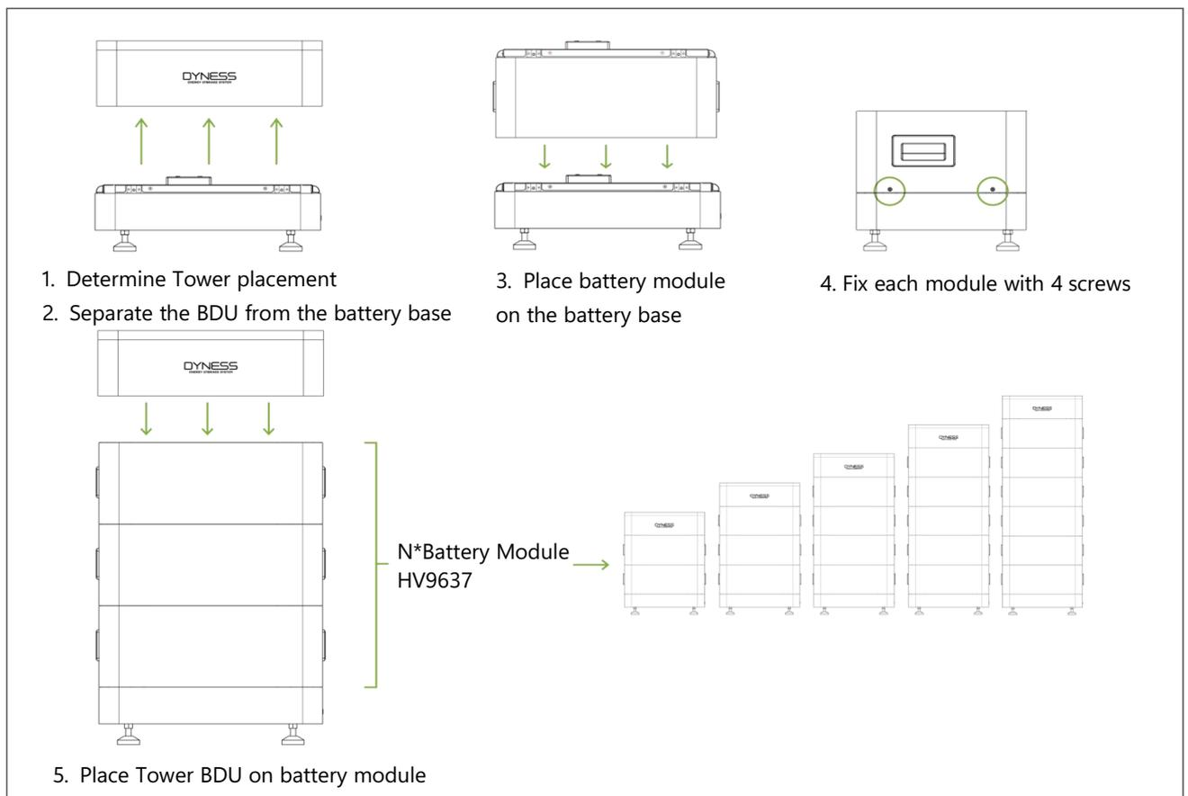
Figure 3-5 Mechanical Installation
