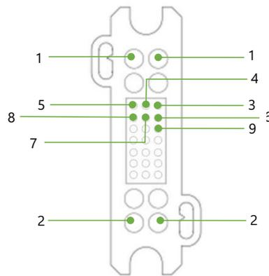
Figure 2-6 Composite Connector-Socket
