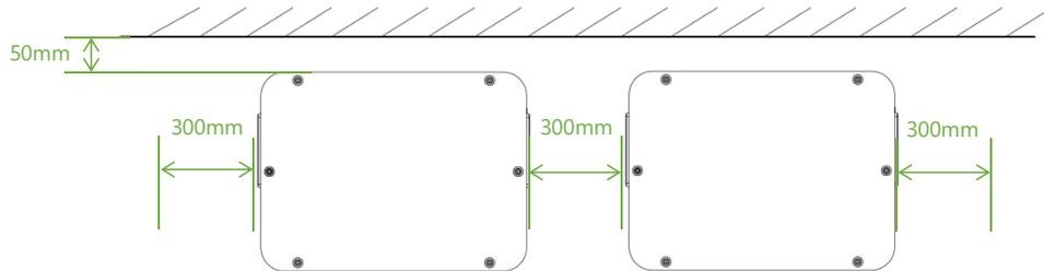
Figure 3-1 The Minimum Clearance Diagram
